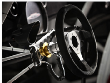
Figure 9 – FDM gauge pod endures five-G impact forces.
