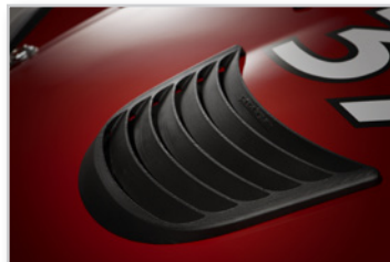
Figure 10 – Adding louvers for style posed no challenge since FDM eliminates tooling.
