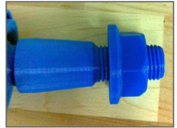
*The Dimension 3D Printer can machine precise threads and grooves using durable FDM, suitable for making functional parts like this bolt assembly for Northstar Manufacturing.*
